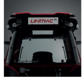
Upon request, powerful H7 halogen or LED working lights are also available. For urban applications, highly visible LED warning beacons and flashing light strips are used. In order to call attention to special operations, LED flashing light strips are employed which can be integrated perfectly into the TracLink roof shell - without negatively affecting the overall height.
